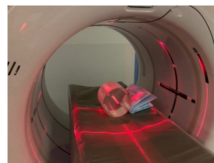
Phantom positioning for localizer and selection of the acquisition box
